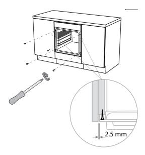
Fig. 4 Securing the oven to the cabinetry
